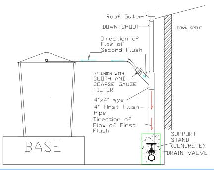
Figure 19 Alternative design for up-flow filter and first flush diverter (using 4" fittings)
