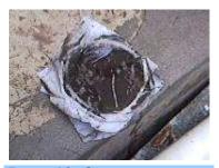
**Figure 18** Contamination residue on the first-flush cloth filter
