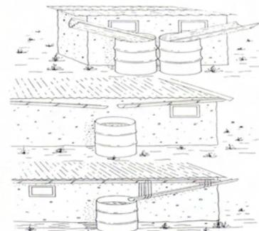
Improvised rainwater collection with 200 l. oil-drums used for storage.
