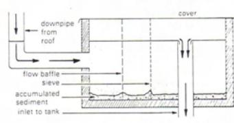
Baffle tank ( 10 litres ) to hold back debris
