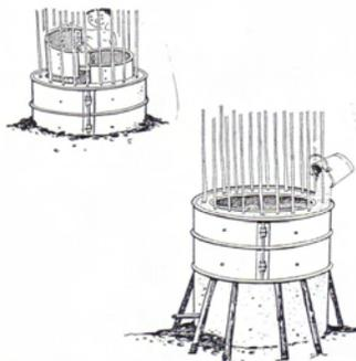
Cast concrete ring tank.
