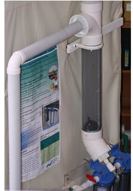
Model first flush (with transparent first-flush section)
